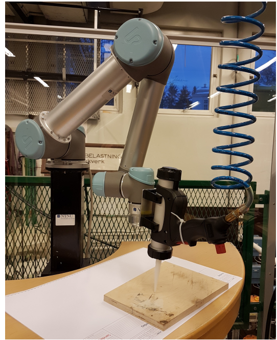
Fig. 6. Experiment set-up: A caulking gun driven by compressed air is connected in parallel to the end effector of a UR-5 robot arm.
