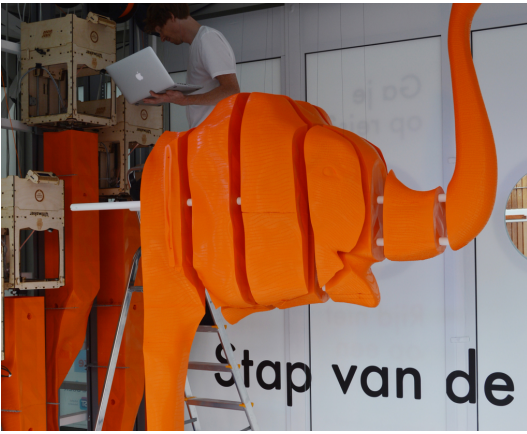
Fig. 1. 3D Elephant Petition: The pieces that make up the 3D-printed elephant sculpture were made by five traditional Ultimaker 3D-printers. Each of these printers were given an extended degree of freedom by connecting them to a rail that moved vertically, which made it possible to print pieces that were up to 2.5 meters tall. Photo: www.rooiejoris.nl [2].
