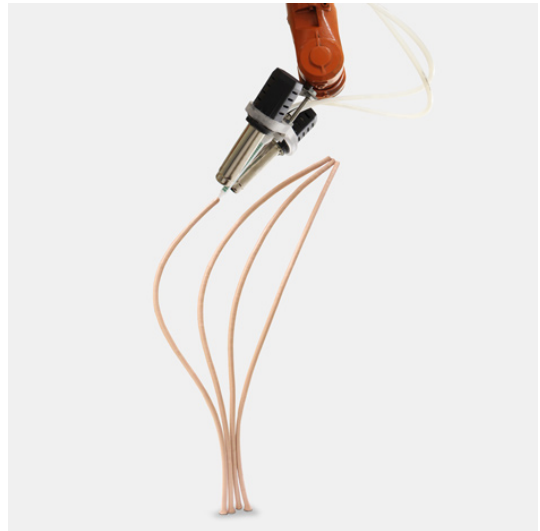
Fig. 4. Mataerial project: Combining an industrial manipulator with a fast-curing plastic makes it possible to "print" double curved lines in mid-air. Photo: www.mataerial.com [21].
