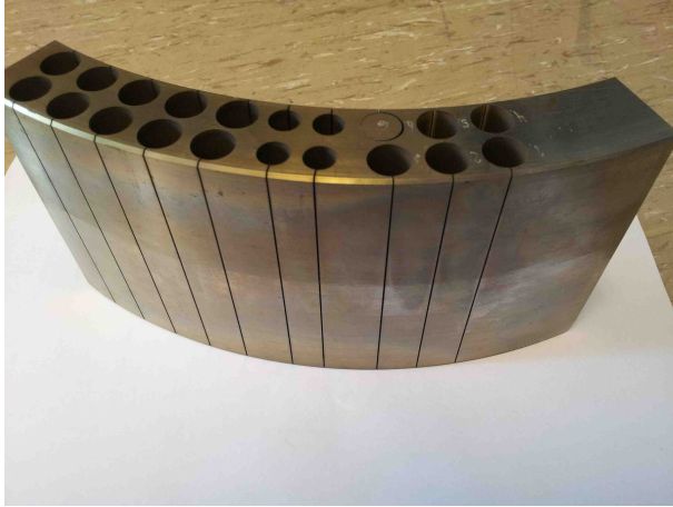
Figure 12: A picture of how the Alloy 725 samples were extracted from the material.
