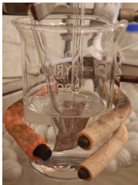
Figure A.2: Setup for making of the reference electrode.
