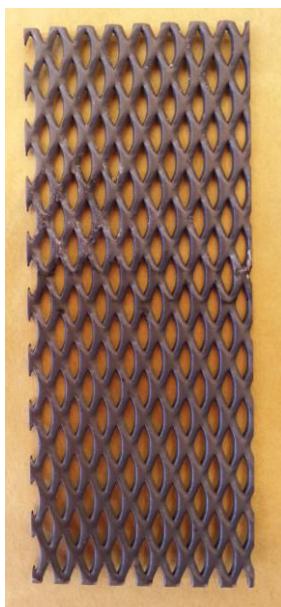
Figure 4.6: RuO 2 /IrO 2 mesh electrode from Permascand (PSC 102).
