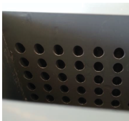
Figure 4.5: Separator of anode and cathode compartment in flow cell.
