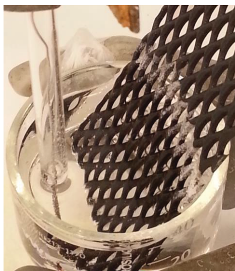
Figure 5.33: Deposit discovered on the working electrode after long time electrolysis in both synthetic electrolyte and process water.
