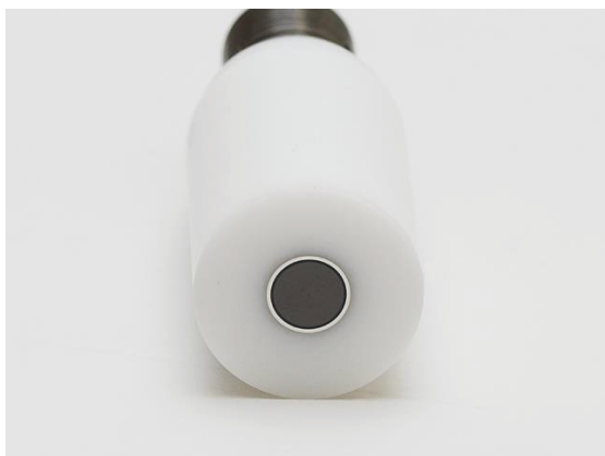
Figure 2.8: A rotating ring-disc electrode (RRDE) [18].
