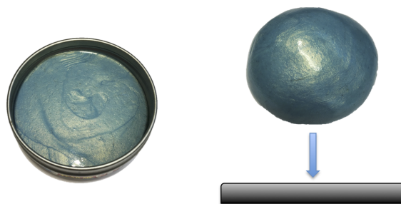
Figure 1.11: Viscous and elastic behavior of silly putty. It will flow to fill a container and when shaped to a sphere and thrown it will bounce back.
