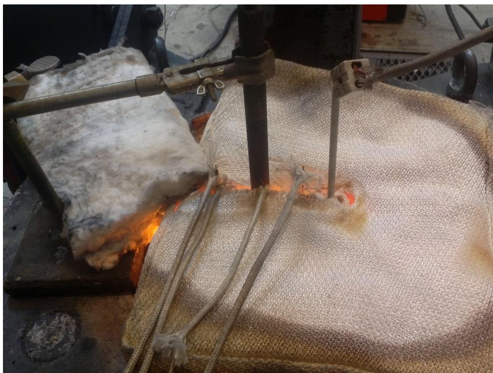
Figure 3.6: Top of furnace during experiments. To the far right is the thermocouple and in the centre a graphite lance is seen.
