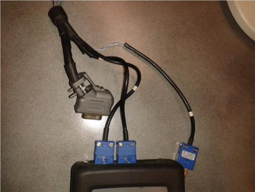
Figure 23: Connect cable marked 1 and 2 in the thermometer.
