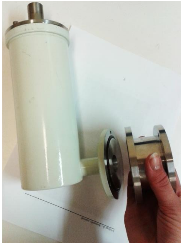
Figure 16: Screw the upper door contact to the liquid nitrogen container.
