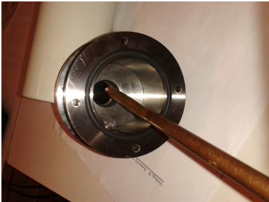
Figure 18: Screw the cold finger to the liquid nitrogen container.
