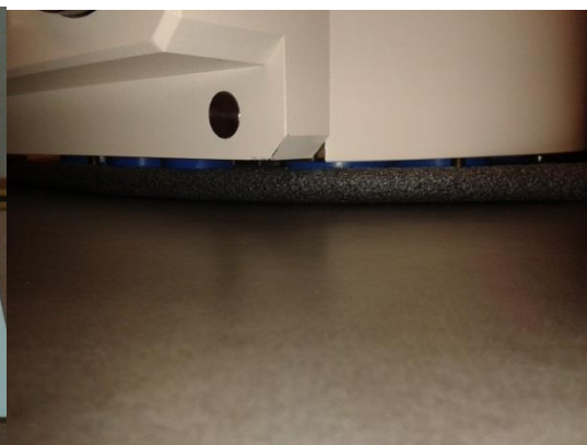
Figure 2: Shred of foam rubber placed under the SEM
