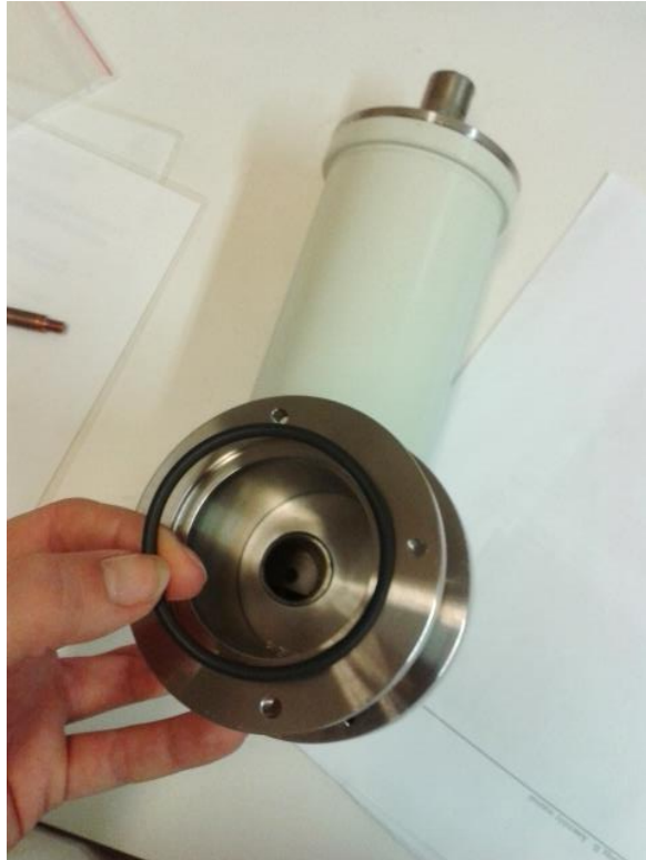
Figure 17: Place the gasket on the other side of the upper door contact
