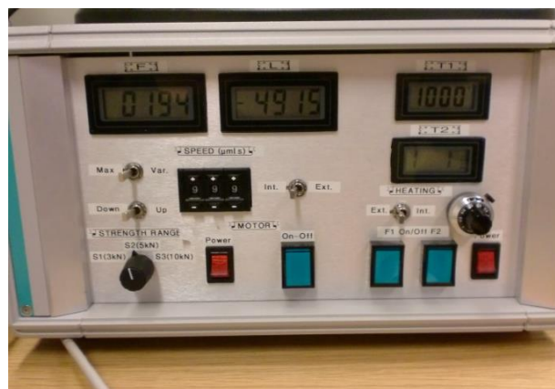
Figure 14: This is how the tensile stage control box look like when you have executed step 1-4.
