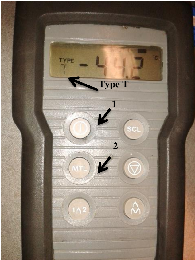
Figure 24: To start the thermometer, press button 1, and then button 2 until the display shows "Type T"
