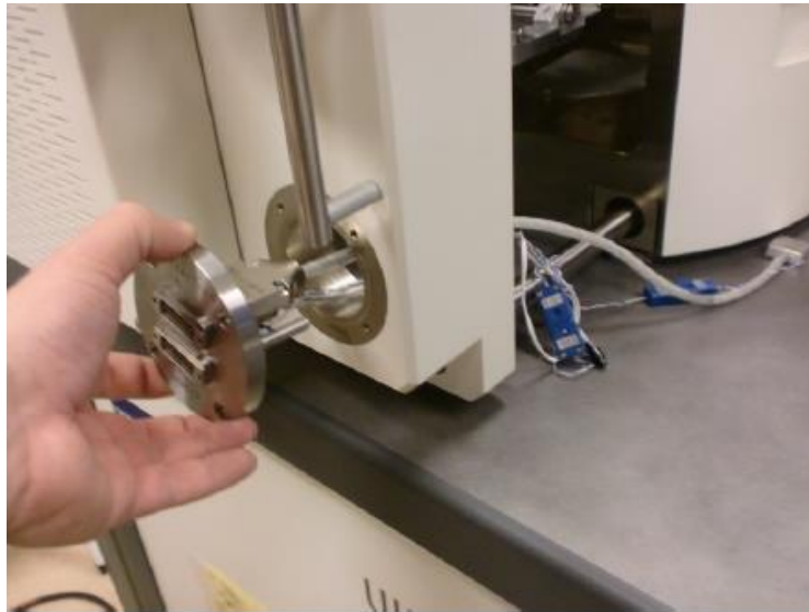
Figure 11: Mount the traction cable and the thermocouple to the door contact, lead the cables through and screw the contact to the door. Use the screws from the original door contact.
