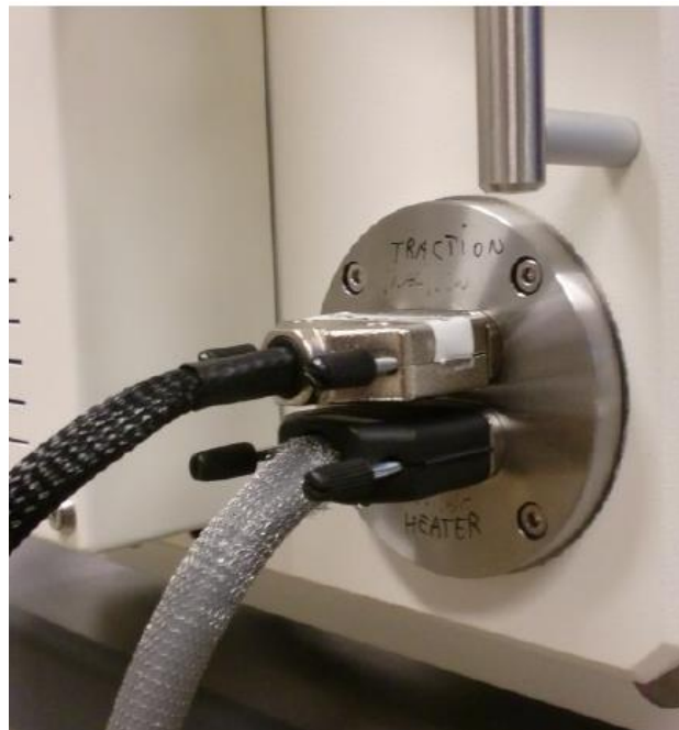
Figure 12: Connect the cable from the moveable computer. Traction cable in upper contact and thermocouple cable (part X from figure X) in the lower contact.
