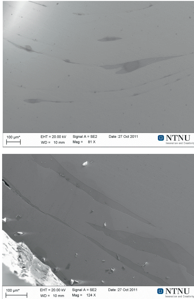
Figure 4.38. SEM micrographs of the screw extruded macrocomposite; (a) close to the center of the cross-section, (b) close to the end of the cross-section, i.e. the outer surface of the rod.
