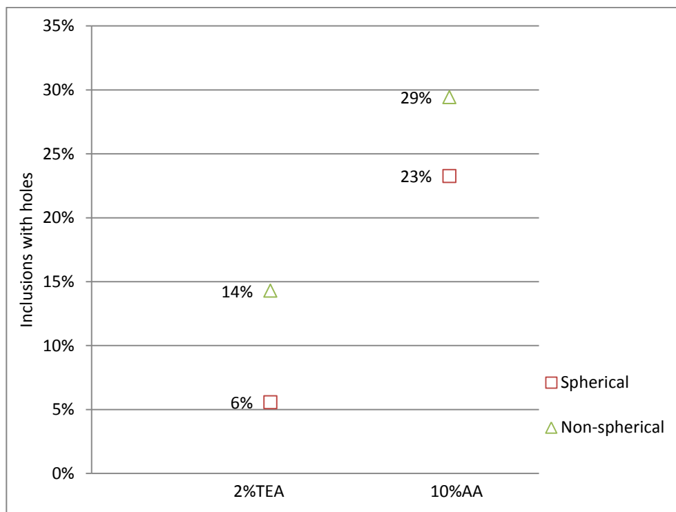
Figure 22: Morphology distribution of inclusions in 2% TEA and 10% AA electrolytes
