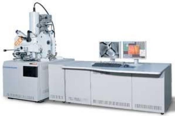
Figure 3.3 EPMA instrument JXA-8500F
