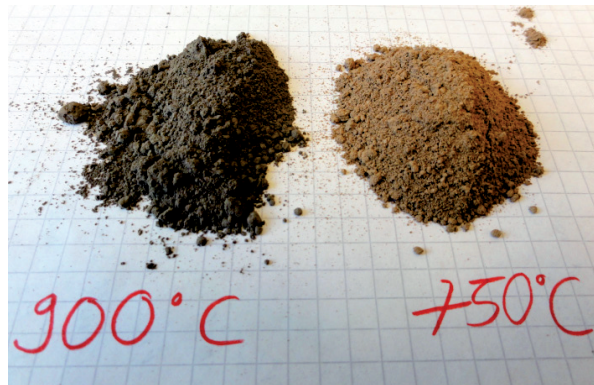
Figure 7-5: Calcined Clays at 900 and 750 °C (measured temperature at kiln outlet)
