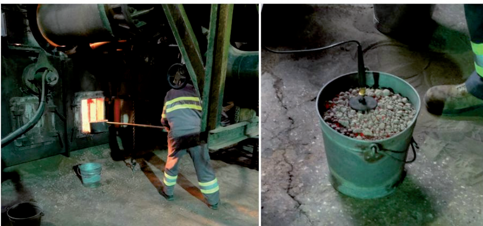
Figure 7-11: Employee taking out material from the kiln head (left) and measuring temperature with a thermocouple inside the material (right)
