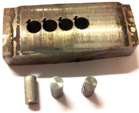
Figure 28: Pin samples cut out from a tool joint section.
