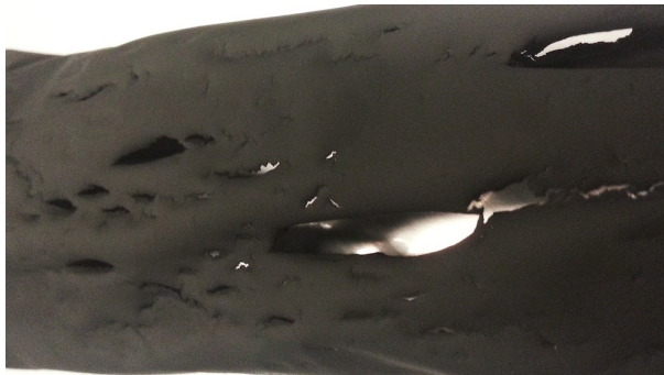
(a) Green tape of LSFTa porous support casted with the slip specified as Tape 1 in Table 3.9. 16.7 vol.% solid loading. The tape curled up and cracked during drying.
