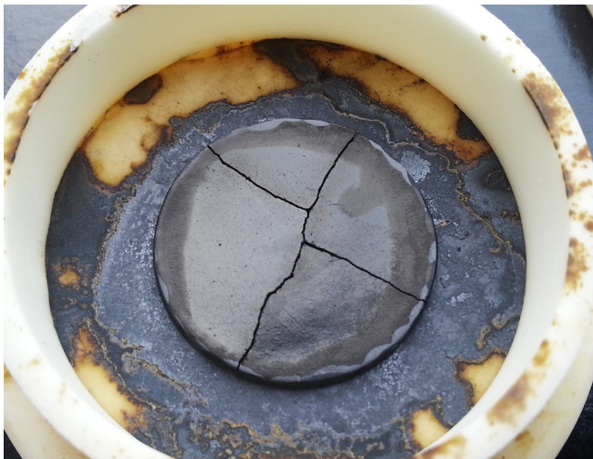
Figure 4.33: Picture of the LSFAl porous support pre-sintered at 1200°C. The support cracked while being immersed in the dip coating suspension.
