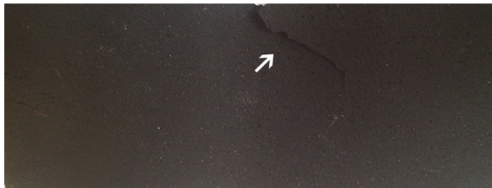
Figure 4.30: Dried tape casted from the LSFAl slip prepared following the same procedure as for making LSFTa tape casting slip, specified in Figure 3.1. The slip was heavily coagulated and the casted tape was very weak. The arrow highlights a crack.
