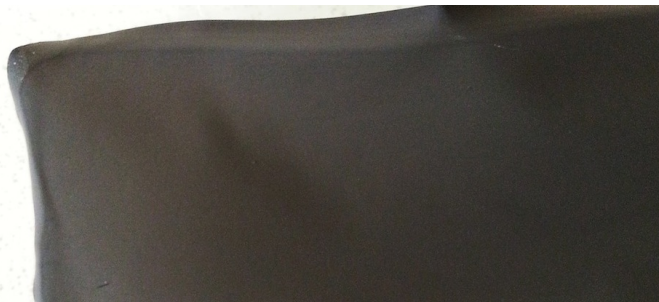
(b) Green tape of LSFTa porous support casted with the slip specified as Tape 2 in Table 3.9. 15.8 vol.% solid loading. The tape was homogeneous, nearly flat and very flexible.
