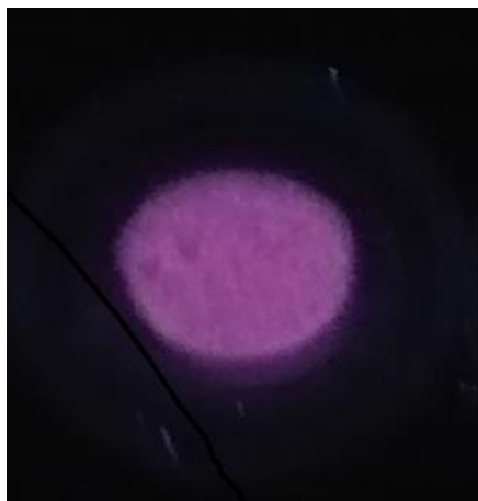
Figure 4.13: Calcined M-75-30-Eu under exposure to ultraviolet light with wavelength 366 nm.
