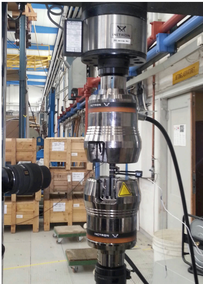
Fig. 3-7: The machine used for the upsetting testing, an Instron 8032. A camera setup was used to record test images every 10 seconds, and an extensometer was used to measure the displacement during the compression.
