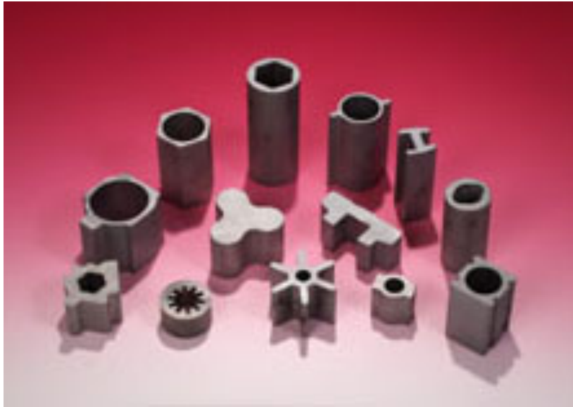
Fig. 2-2: Examples of extruded materials showing the complexity of the extruded shapes[12].
