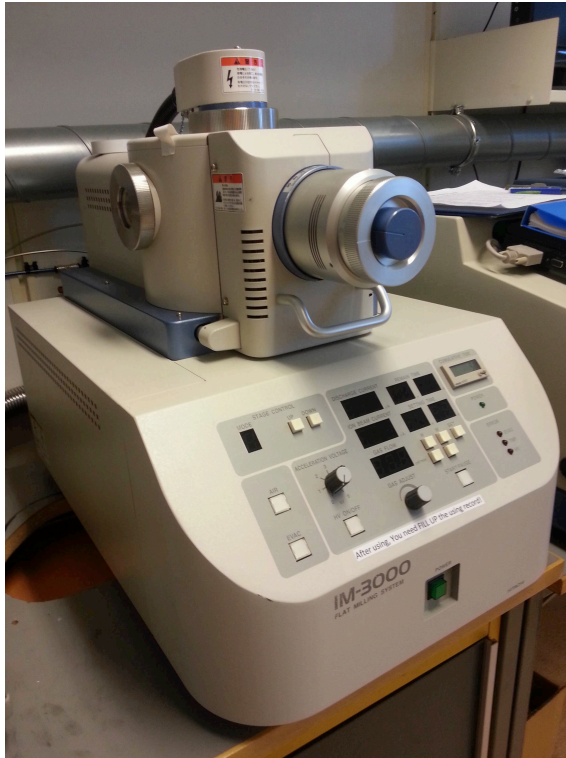
Fig. 3-4: The ion milling instrument used in the present work, an IM-3000.
