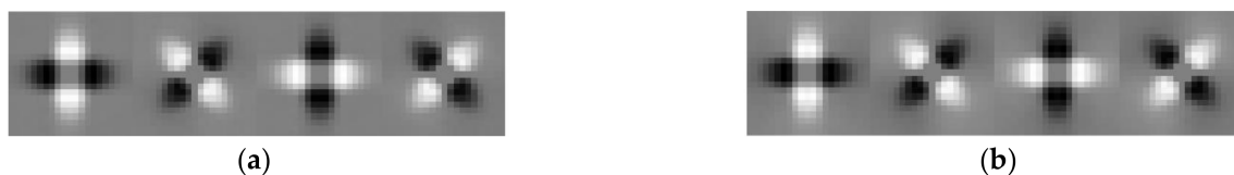
Figure 9. Equivalent feature extractors t_\theta(m,n) of the old PCA-based detector [14], for orientations \theta \in \{0^\circ, 45^\circ, 90^\circ, 135^\circ\} , in the Cx channel (a) and Cz channel (b).
