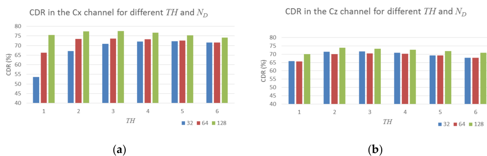
Figure 6. CDR for all images and capture devices using dictionary-based detector, in the Cx (a) and Cz channel (b), depending on the dictionary size N_D (color-coded) and the number of atoms used in the detection TH .
