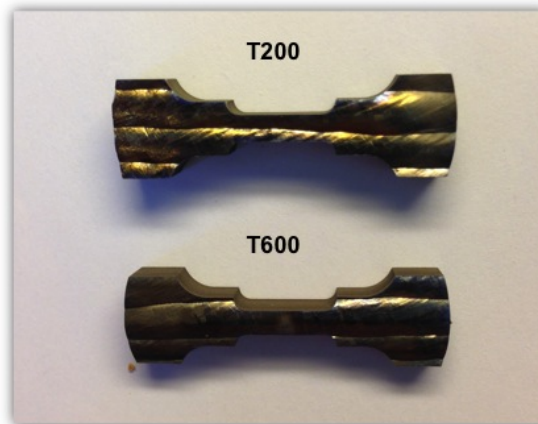
Figure 32: The T200 specimens contains two deposits, while T600 only contains one. This is expected to give microstructural variations between the specimens.
