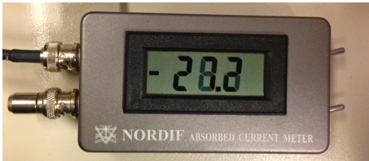
Figure 27: The NORDIF Absorbed Current Meter used to calculate the probe current in the Hitachi Microscope.
