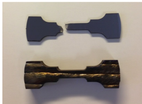
Figure 64: Specimen T200 after failure
