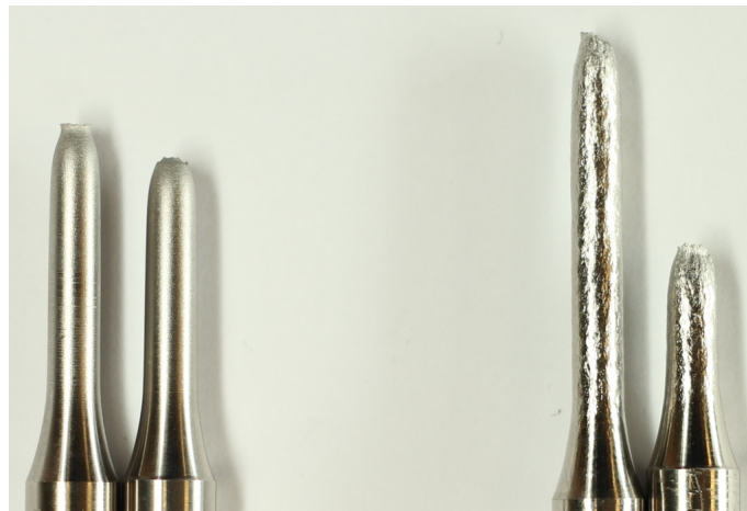
Figure 4.3.1: The image show samples from the tensile testing. Sample from HIP material is to the left and from the forged material is to the right.
