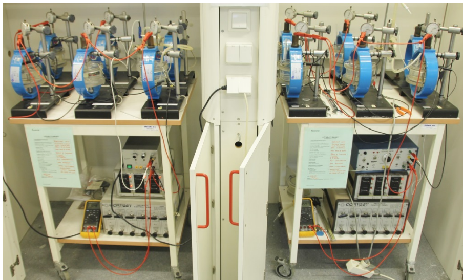
Figure 3.3.3: Image showing the equipment used for HISC testing.
