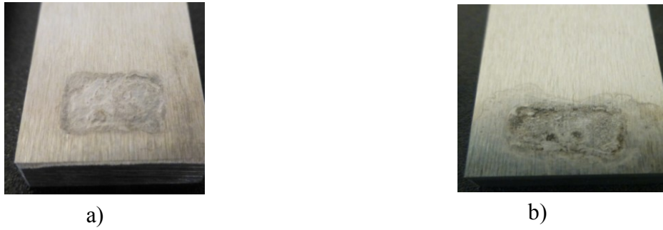
Figure 4-28. Corrosion of steel samples after testing for one week at a) 80 \text{ A m}^{-2} and b) 100 \text{ A m}^{-2} .
