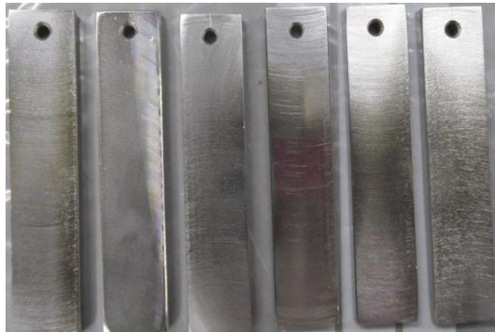
Figure 8: Prepared samples cleaned by grinding before coating
