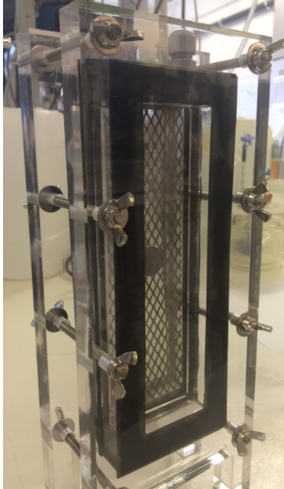
Figure 1.2: Anion exchange membrane module
