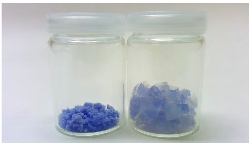
Figure 4.4: Picture of dried gels straight from the drying furnace with samples containing the same weight. Unwashed gel to the left (Co0.0125) and washed gel to the right (Co0.0125_W).
