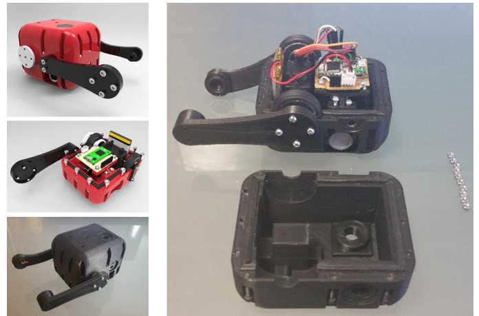
Fig. 3. Final design and 3D printed module
