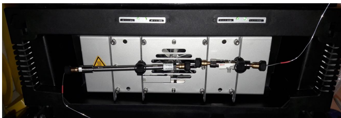
Figure 48: Column compartment of the UHPLC instrument
