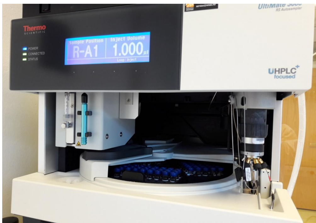
Figure 47: Sampler compartment of the UHPLC instrument
