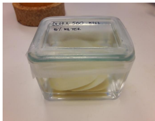
Figure 14: Pre-conditioning of three flat sheets from DuraMem 500 in feed with 90 wt% EtOH
