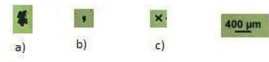
Figure 3.1.4: Definition of the defects: a) large defect, b) small defect, c) cross-shaped defect.
