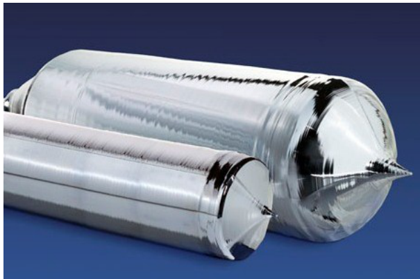
Figure 1.2.4: Two complete Czochralsky monocrystalline ingots with the crown on the right hand side, and the tail on the left (19).
