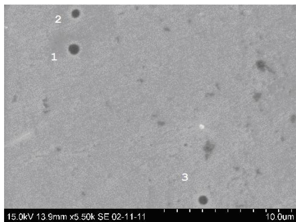
Figure 24 Inclusions in Base Metal Sample 2 before electrochemical polarization.
