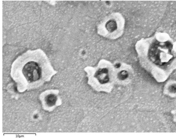
Figure 51 Inclusion-like formations in Weld Sample 3.
