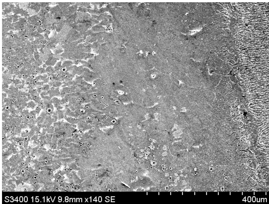
Figure 47 HAZ between 0 mm (to the right) and 0.8 mm from the fusion line in Weld Sample 3.
