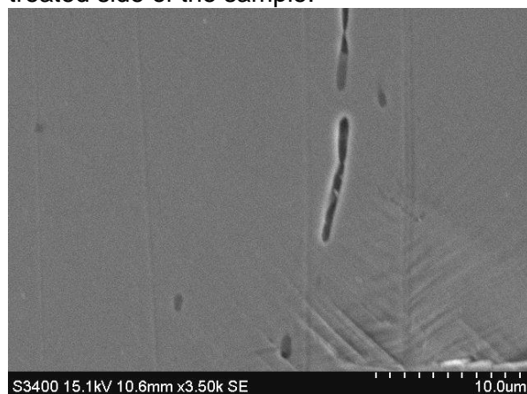
Figure 13 Inclusions at 16 mm from the fusion line after welding, on the side of the weld sample not treated with acid.
