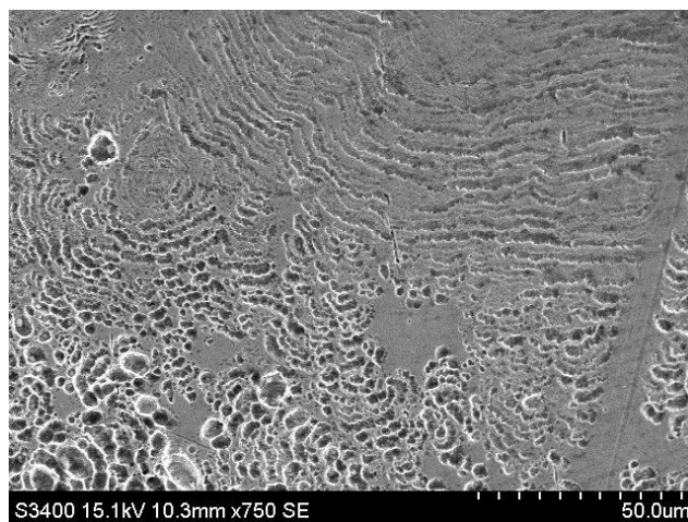
Figure 35 Close view of corroded area in Weld Sample 1a.
