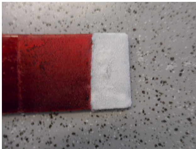
Figure 4.1: Calcareous deposits on carbon steel
