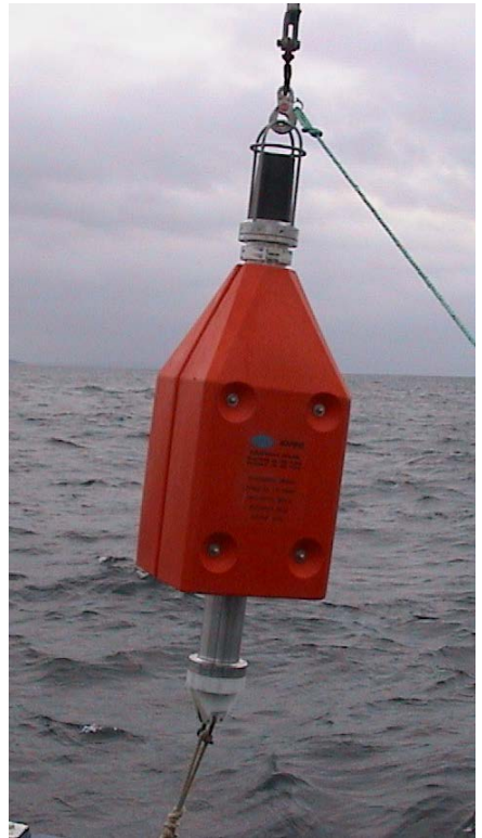
Fig. 8. Left: HUGIN 2D trajectory in UTP sea trial. UTP was deployed at x = -396 m, y = -151 m (relative coordinates). Right: Underwater transponder used in sea trial.
