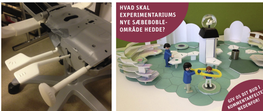
Figure 4 Example of a low-functional prototype used in the stages after concept development. From the left 3D printed handles used by Scandinavian Business Seating (prototype no. 6) and a small scale model of the future soap bubble exhibition at Experimentarium (prototype no. 13)
