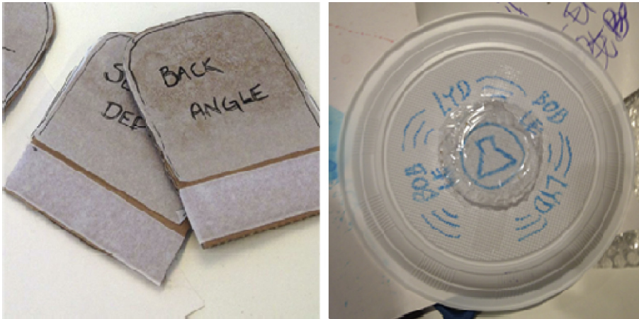
Figure 2 Example of low-functional prototypes used in the concept stage. From the left prototype handles of cardboard used by Scandinavian Business Seating (no. 4) followed by prototype no. 11, communicating the idea of a soap bubble being affected by the vibration of sound.
