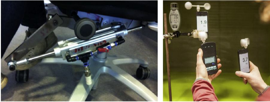
Figure 5 Example of high-functional prototypes used in the stages after concept development. From the right, hydraulics test used by Scandinavian Business Seating (prototype no. 5) and Vaavud testing fluid mechanical properties in a wind simulator (prototype no. 15)
