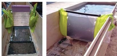
Figure 3 - First experiment setup of investigating sealing performance
