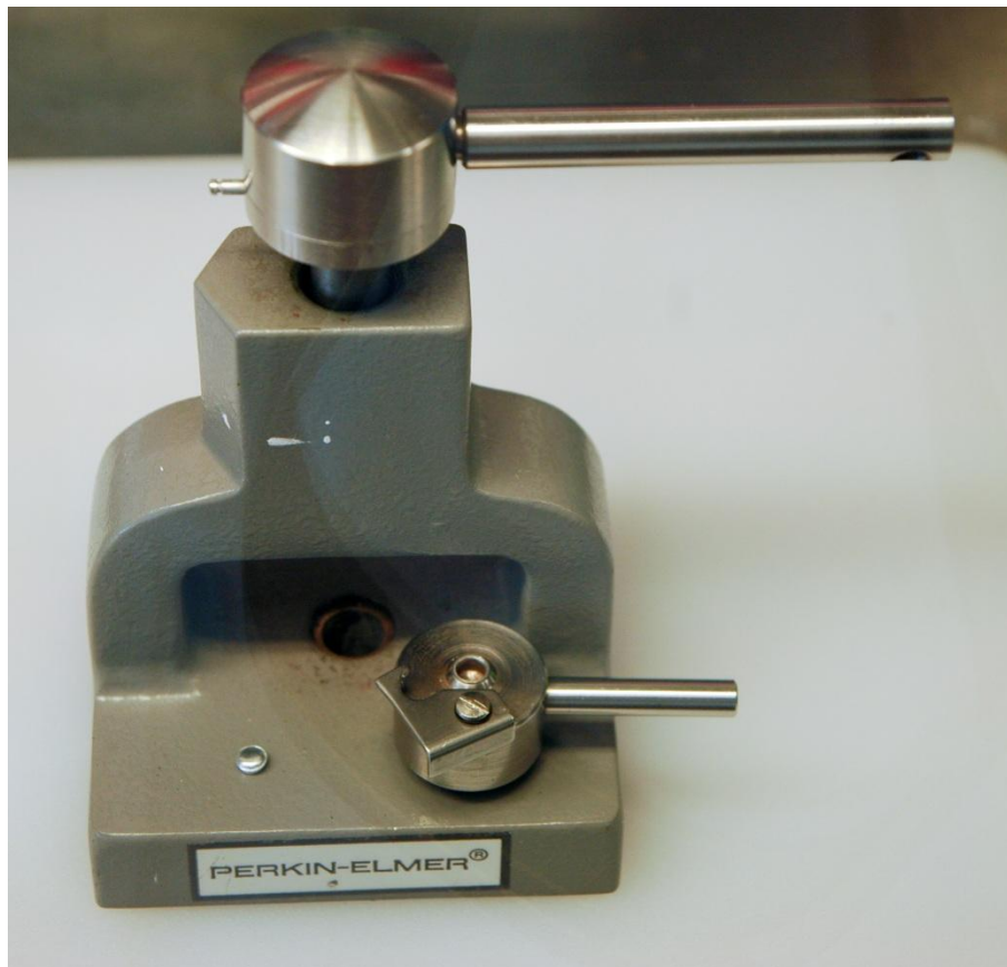
Figure 22: Sealing tool for the aluminium sample pans for the low temperature DSC analysis. A sealed pan is placed on the tool platform to the left of the pan holder.
