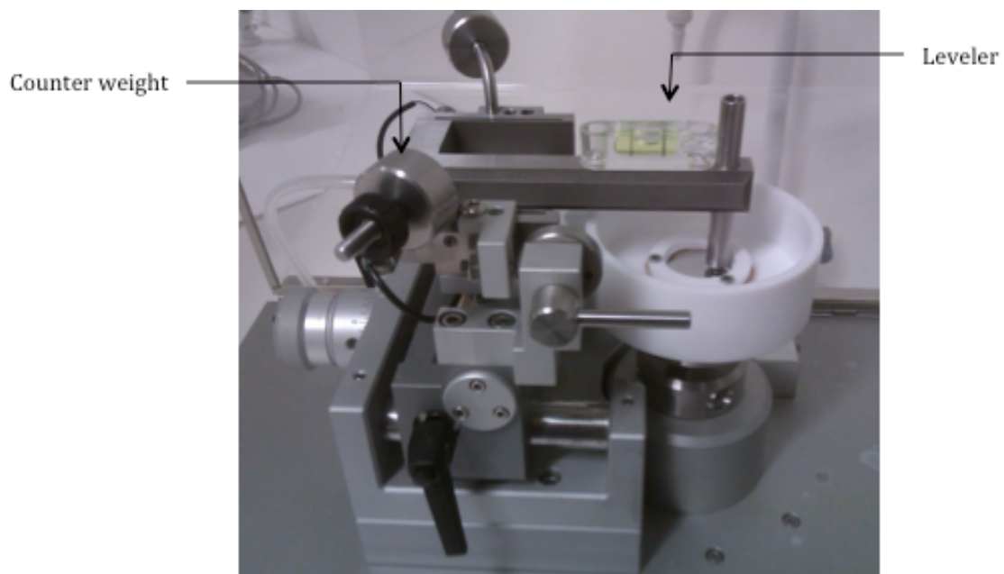
Figure 3.2: The leveler and the counter weight
