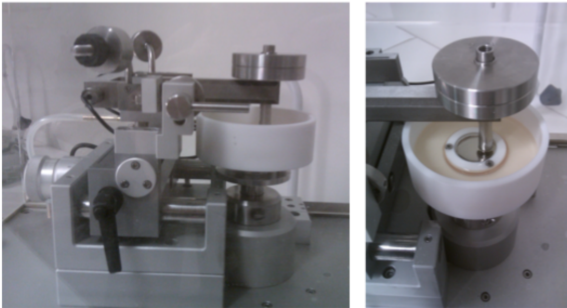
Figure 3.3: Pin-on-disk apparatus ready to use
