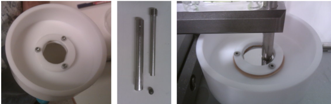
Figure 3.1: Images of the sample mounted in the Teflon holder (left), the ball and the ball-holder (middle), and the ball in contact with the disc
