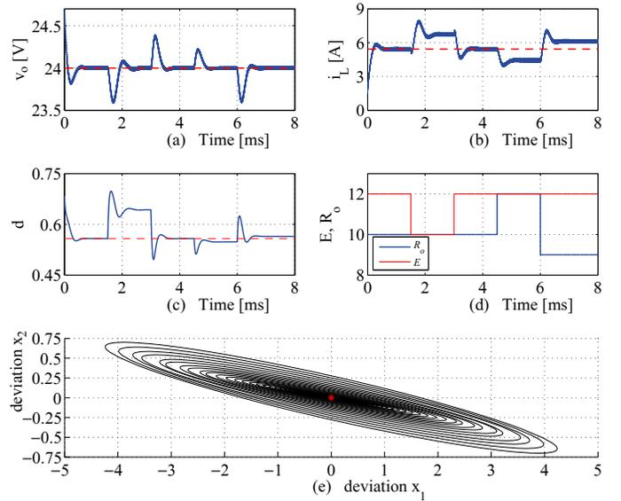
Figure 3. Simulation results for the boost converter: (a) output voltage, (b) inductor current, (c) duty cycle, (d) source voltage and load resistor, and (e) region of convergence.
