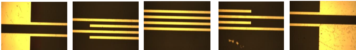
Figure E.3: The electrode area after a successful lift-off process. The metal outside the electrodes is removed.
