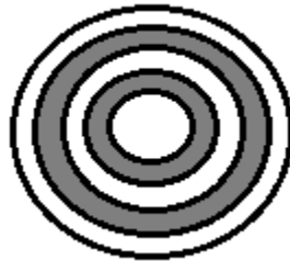
Figure 2.15: A sketch of the hypothetical rotating ring-ring-disk electrode. The grey parts are insulating areas, and the white areas are the disk electrode and the two ring electrodes.
