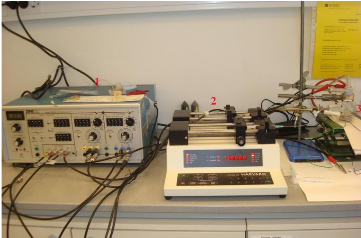
Figure 4.1: Experimental setup. The MFFC (3) is connected to a syringe pump (2) and an analog bipotentiostat (1).
