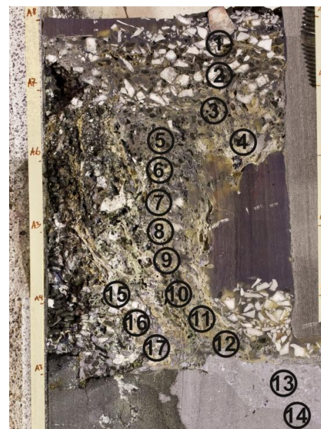
Figure 3.2: Sample extraction from the pilot scale experiment. The cross-section was taken from the side of a quarter piece cut from the furnace.
