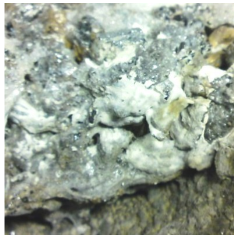
(b) Condensate turned white in crucible 4. T_{bottom} > 1680\text{ }^{\circ}\text{C} .
