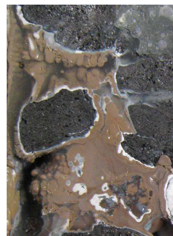
(b) Brown and white condensate formed at \sim 1650 °C.
