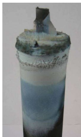
(a) White and blue condensate formed at temperatures between 1100°C and 1430°C.
