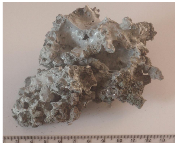
Figure 2.14: Sample taken from the “condensate zone” - raw material held together by condensate. (Tranell et al. 2010)
