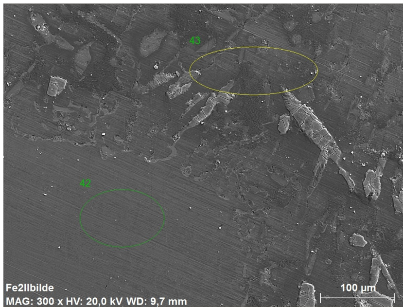
Figure 29: SEM picture of the interface between the two phases in the oxidation experiment
