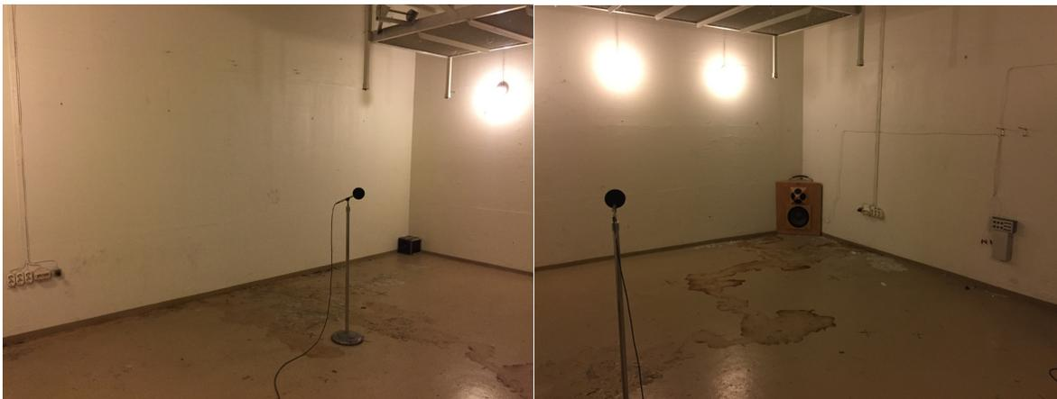
Figure 3.6 Left: The measured absorber. Right: One of the two external sound sources
