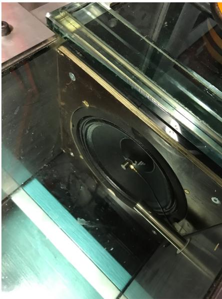
Figure 3.5 Picture of the loudspeaker element with accelerometer and microphone
