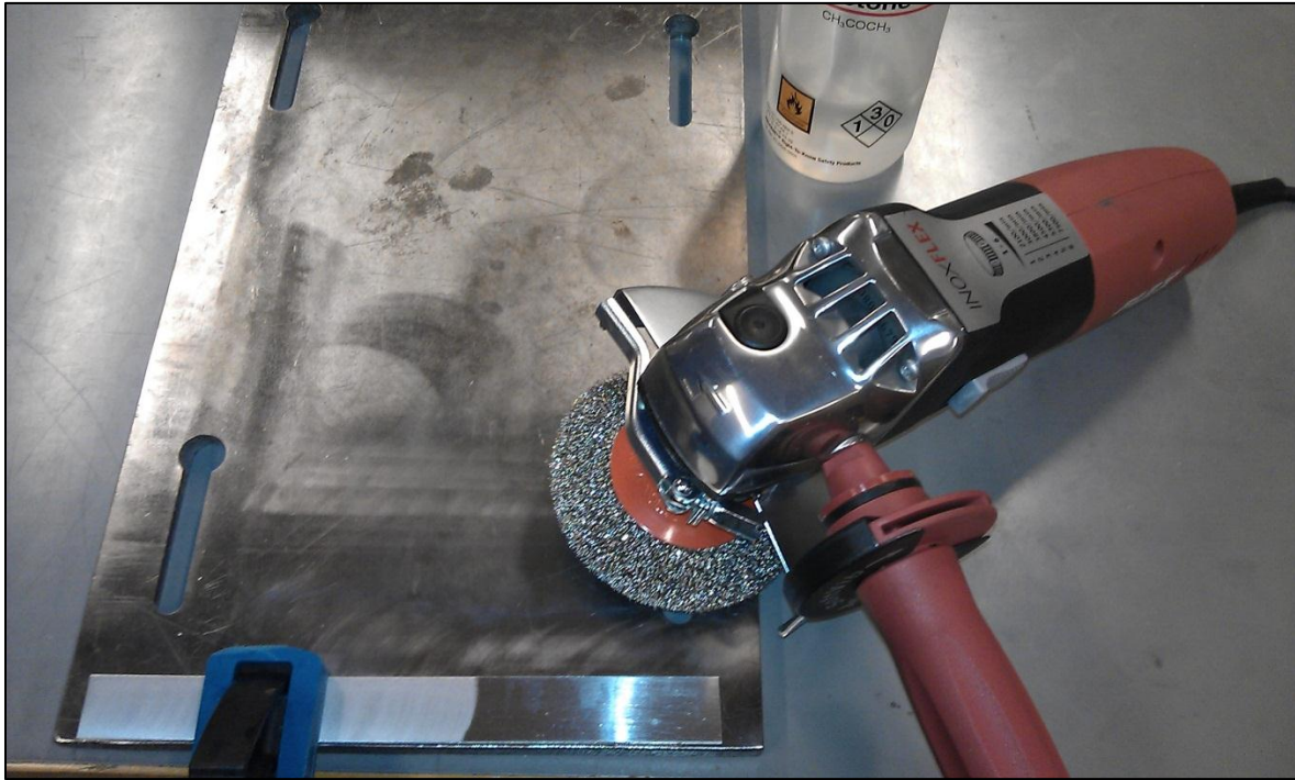
Figure 3.2: Photograph of the wire brushing equipment and a partially brushed aluminum sheet.
