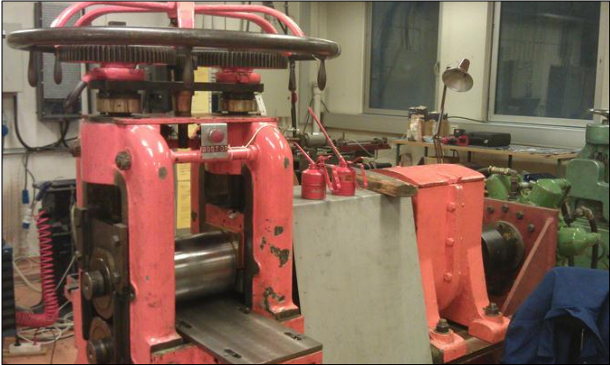
Figure 3.3: The two-high hydraulic rolling mill used for roll bonding.
