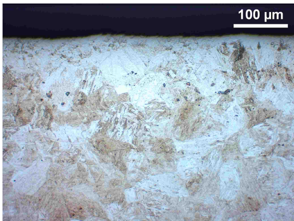
(e) 35M13B, 1000 °C, 15 min, valset side. Avkullingsdybde: 224 µm
