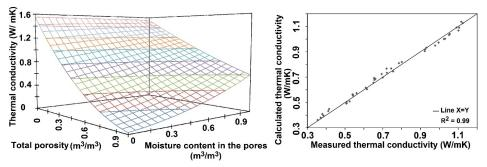
Figure 1 – Thermal conductivity of plain hcps at different total porosities and volume fraction of water calculated from Eq. 1(left), comparison of the measured and calculated thermal conductivities (right)[3]
