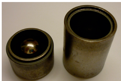
(a) Steel container used to prepare slurry.
