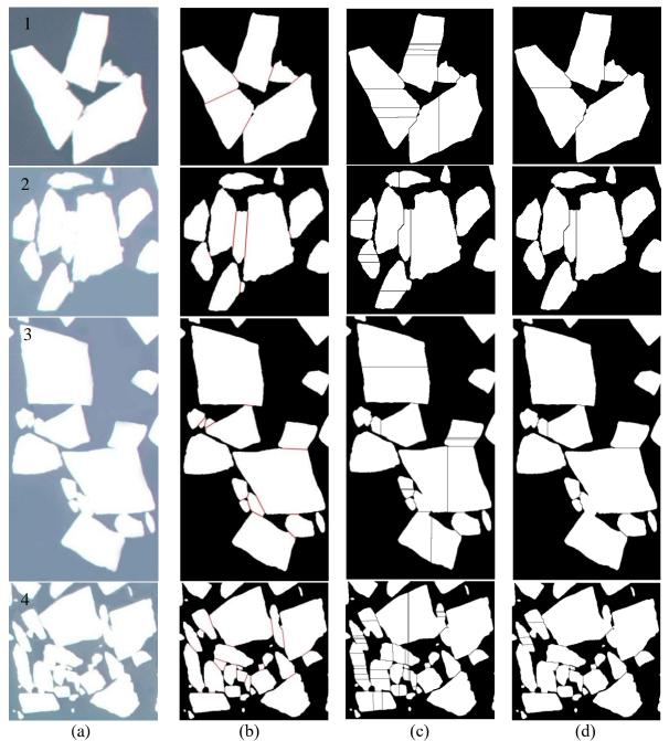
Figure 5. Examples of experimental results: (a) Original ice images. (b) Binary images with manually identified segmented lines between connected ice floes. (c) Segmented images based on the watershed transform. (d) Segmented images after neighboring region merging.
