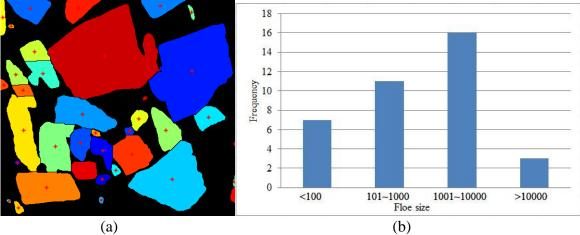
Figure 6. (a) Segmented image with floe center superimposed. (b) Calculated floe size distribution.
