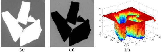
Figure 1. An illustration of some connected ice floes: (a) Grey scale image, (b) its complement, and (c) its topological surface.
