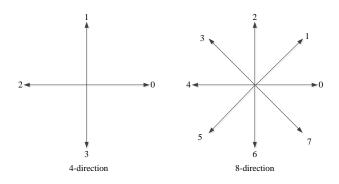
Figure 4. Numbering scheme of the chain code.
