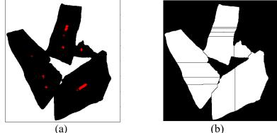
Figure 2. An illustration of watershed-based segmentation: (a) Local minima superimposed in binary image. (b) Over-segmented image.
