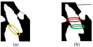
Figure 7. Examples of over- and under-segmentation: (a) Manually identified segmentation. (b) Segmentation by the established algorithm.
