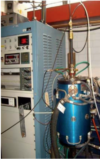
Fig. 3.7 On the left: graphite tube furnace and electrical panel control. On the right: graphite tube containing the charge material connected to a graphite tube.
