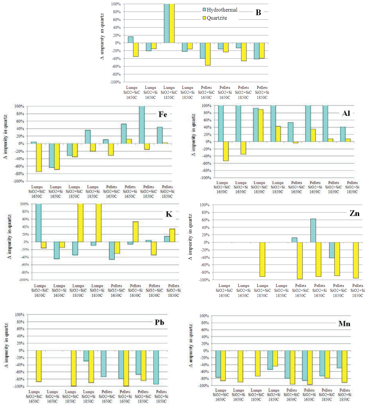
Fig.4- Impurity variation from after quartz reduction compared to the original quartz composition. Values not shown correspond to values below the detection limits or to high concentration in the blanks used as reference.
