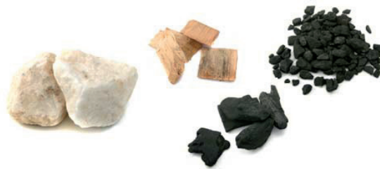
Fig. 1.1 – Common raw materials in the silicon production: quartz, wood chips, coke, coal, charcoal carbon.
