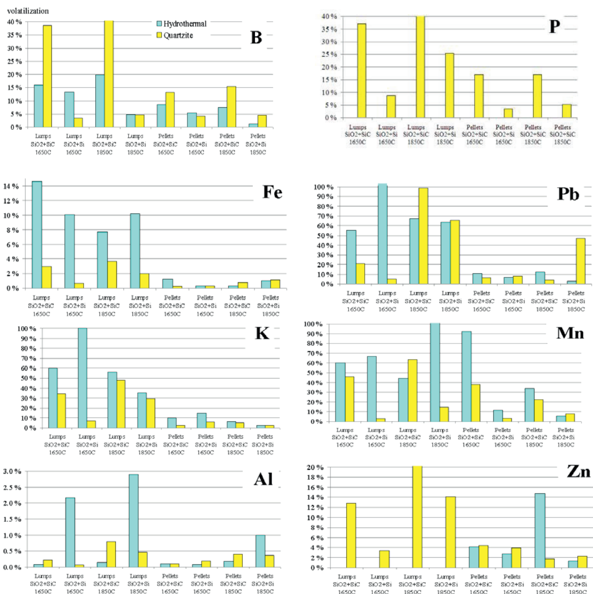
Fig. 6 Volatility of elements (mass %) for different experimental conditions. Note the difference in volatility scale between the individual graphs.
