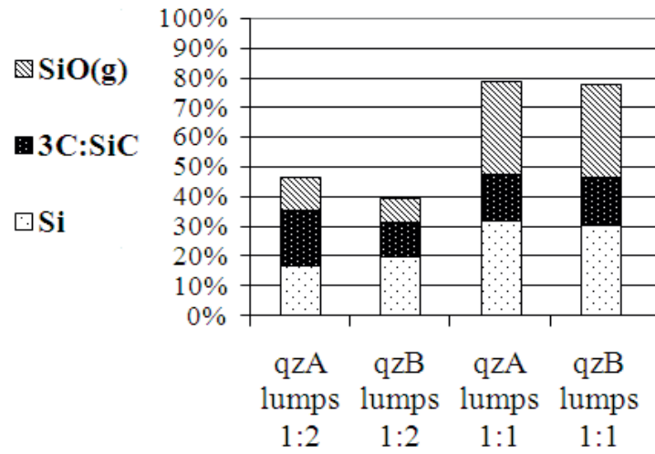
Fig. 4.8 Silicon carbide and two hydrothermal quartzes (qzA and qzB) are respectively heated to 2000 °C in graphite crucibles. Two molar ratios SiO 2 :SiC are considered. The graph plots the total production of SiO(g) with the experimental conditions. Total SiO(g) is due to the contribution of three components: 1) SiO(g) which has reacted with the SiC charge to form Si, 2) SiO(g) which has reacted with the graphite crucible to form SiO(g), 3) SiO(g) which was lost out of the crucible.
