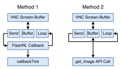
Figure 3: Frame-buffer Access Methods
