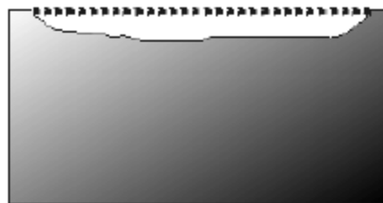
Figure 2.12: Uniform corrosion [54].
