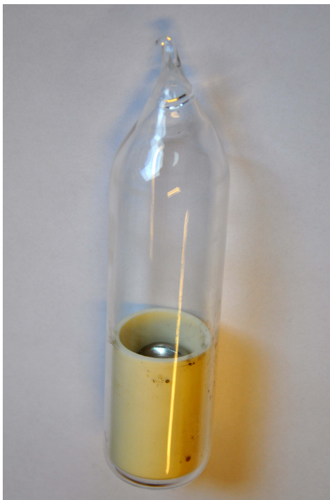
Figure 3.2: Vacuum capsule with alumina crucible inside.
