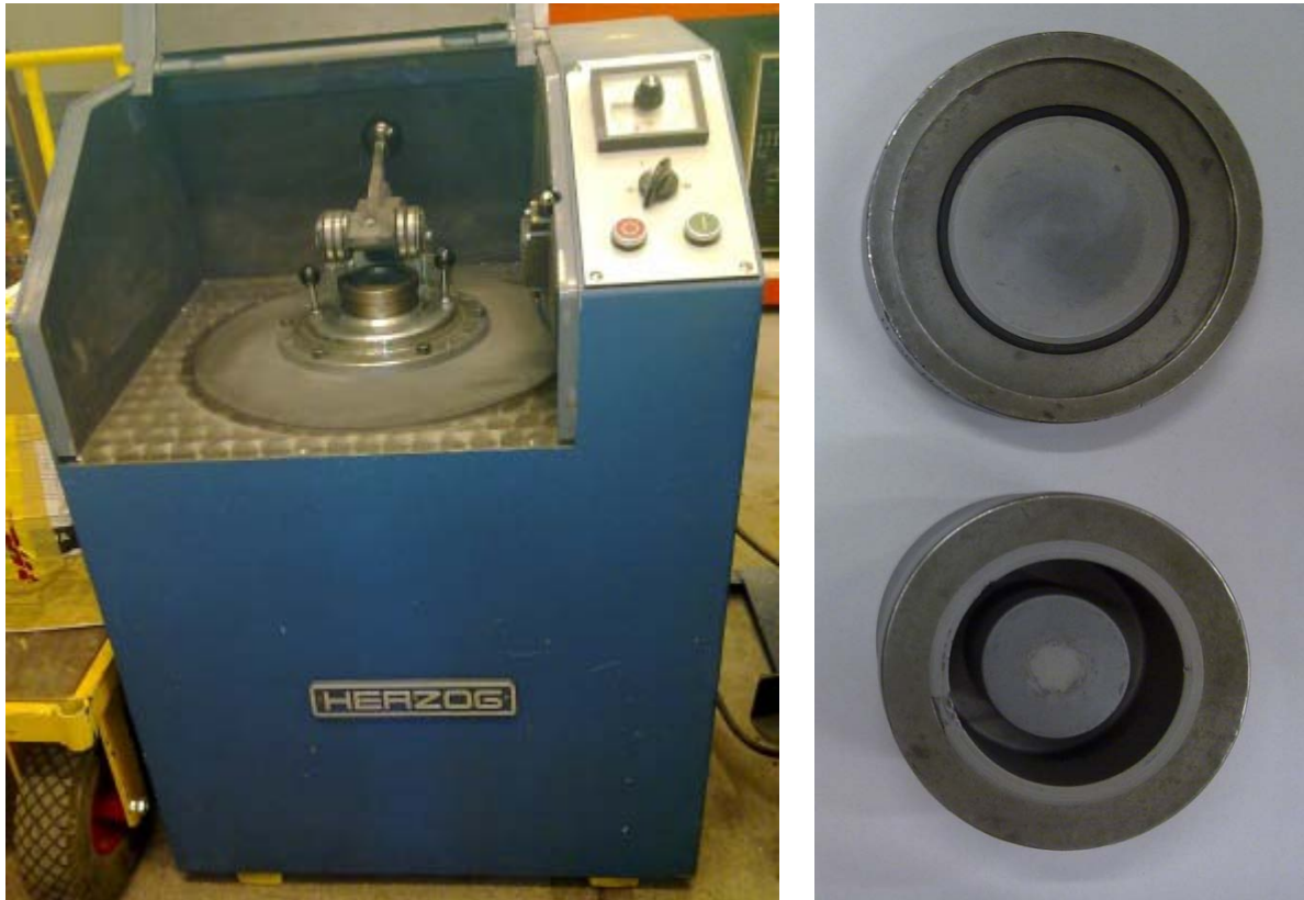
Figure 15: Grinding equipment: grinding mill (left), tungsten carbide grinding head (right)
