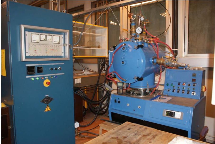
Figure 11: General view of the vacuum induction furnace facility set-up
