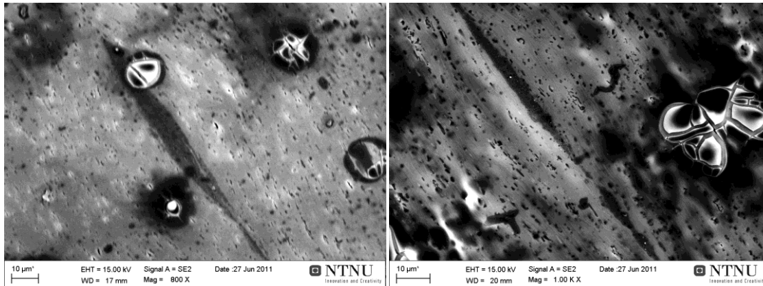
Figure 48: Sample A2NA02 observing the bond interface from the side. From the left a 800x and 1000x magnification image of the interface of roll bonded aluminum. The electro polishing for this sample was not fully satisfactory, but the interface is yet clearly visible.
