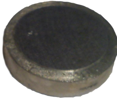
Figure 52: This figure is showing a picture of a sample which split in the metallic bonding during testing. Prior to testing this sample had a groove machined in its side.
