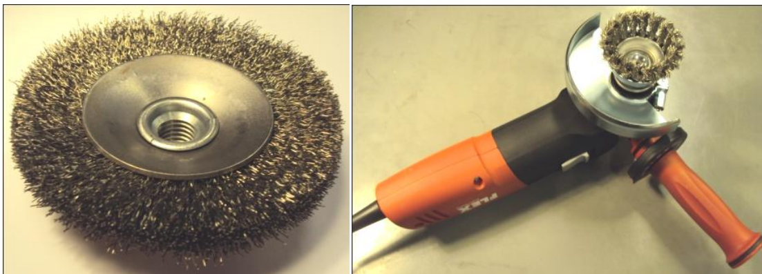
Figure 16: The brush used in these experiments shown to the left, and the grinder to the right.
