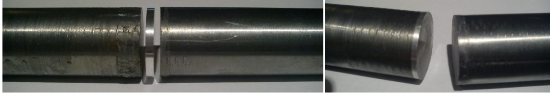
Figure 31: This figure shows how the disc samples are placed between the rods.
