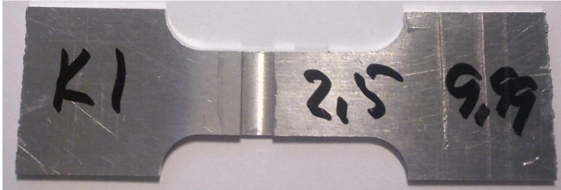
Figure 22: A shear bond strength sample cut and prepared for testing.
