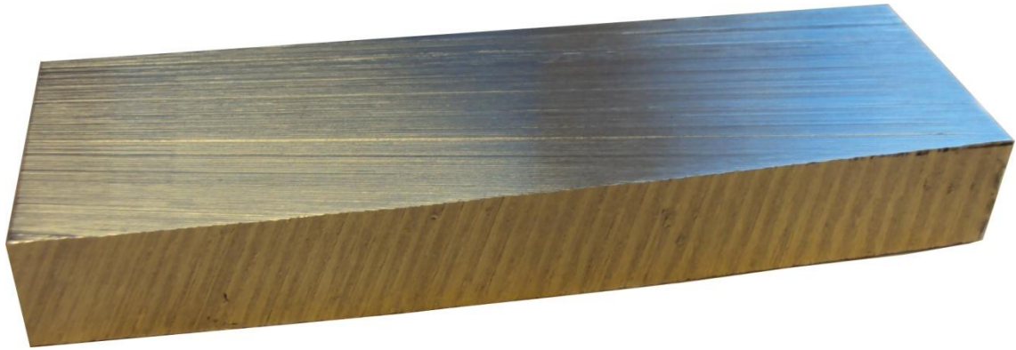
Figure 18: A piece of 3103 aluminum alloy prepared for rolling down to final sheet thickness.
