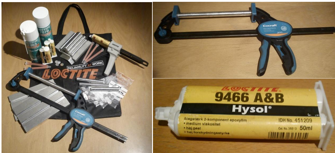
Figure 30: To the left is a picture of the gluing kit shown and to the right a sample clamped between two rods and a close-up of the glue used.
