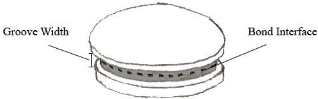
Figure 25: A sketch showing where the groove was cut to reduce the bond cross-section.
