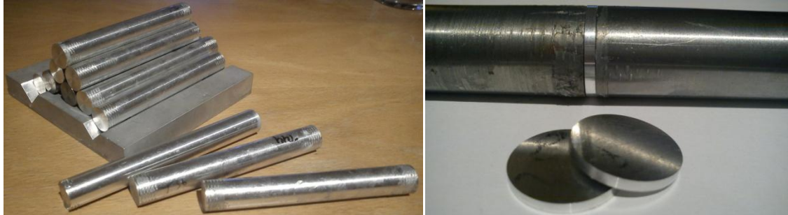
Figure 29: To the left is a stack of the aluminum rods used to test the disc samples. On the right side is one of the samples fitted in-between two of the rods.
