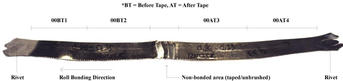
Figure 32: This figure shows how to intertid the appellations of the peel-test samples. [10]
