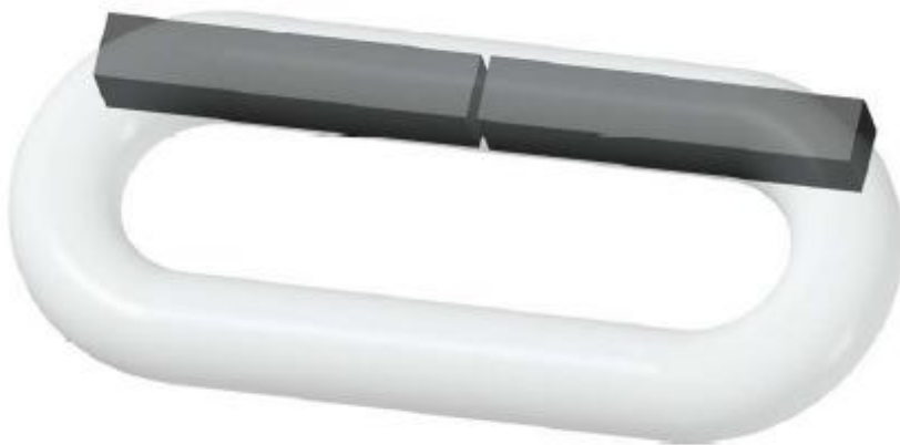
Figure 16. The sketch shows the positioning of the Charpy samples in the chain ring. Here from the welded side of the ring.
