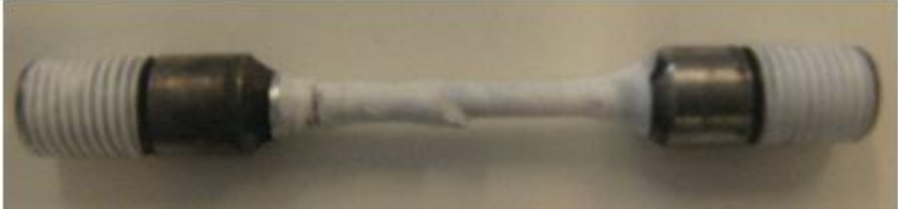
Figure 42. Picture displaying the masking of the HDG tensile specimen before it was etched.
