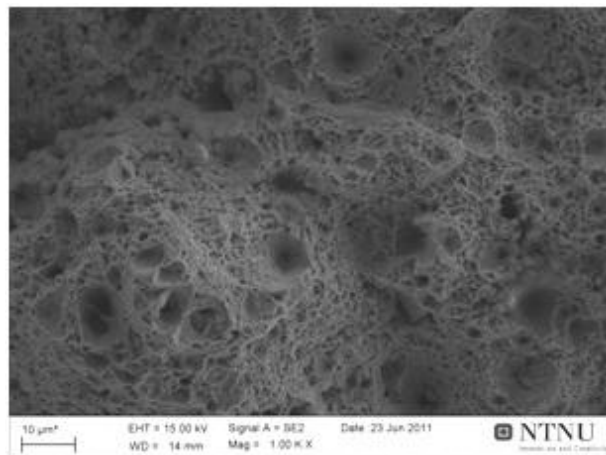
Figure 49. a) Macroscopic view of the tensile specimen CorTest15.s of the fractured chain at 25x. b) Fractographic photo of the center of sample CorTest15.s at 1000x with dimples.
