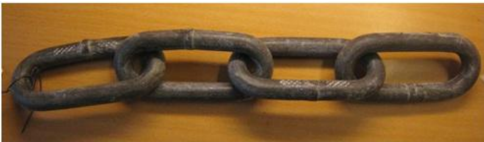
Figure 13. The link of the fractured chain steel as-delivered.
