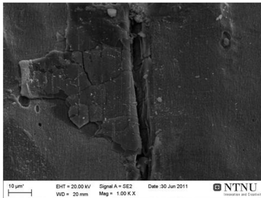
Figure 39. Surface examinations of specimen CorTest7.s(free) in the SEM at; a) 25x, b) at 1000x the center of the sample.
