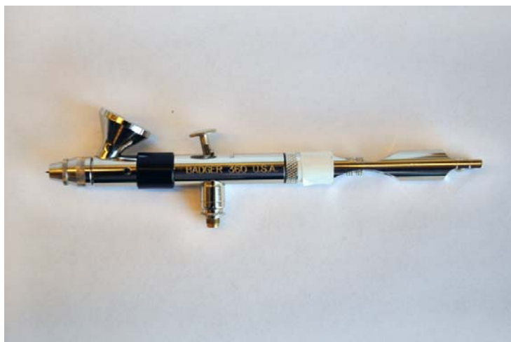
Figure 3-1 air brush used for spraying the catalyst
