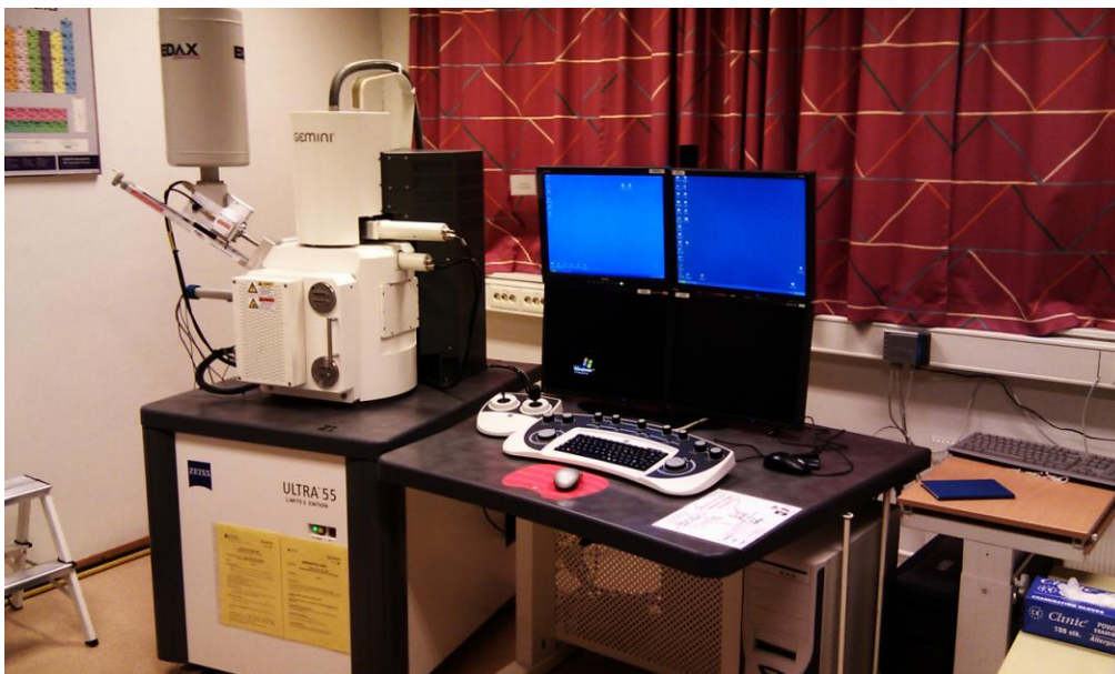
Fig. 3.17: Zeiss Ultra 55 – Limited Edition FESEM equipped with an EBSD-detector
