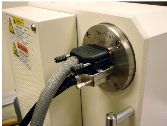
Figure D.20: Cables from hot stage controller and temperature logger connected to the SEM.
